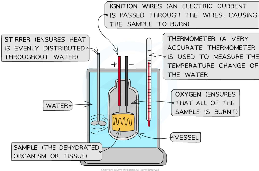
**An example of a more precise (and much more expensive) version of a calorimeter known as a bomb calorimeter - this type is used in professional scientific laboratories**
